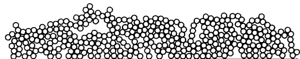
Figure 8 Final stage of simulation, Run 5. Simulation conditions: 0.4 packing density, 0.01 sticking probability, 10 pixels amplitude and 200 pixels to aggregate.
