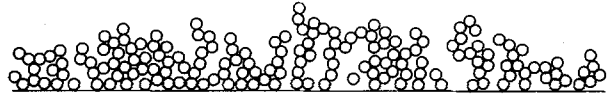
Figure 18 Final stage of simulation, Run 15. Simulation conditions: 0.2 packing density, 0.01 sticking probability, 1 pixel amplitude and 200 pixels to aggregate.
