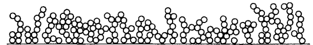
Figure 19 Final stage of simulation, Run 16. Simulation conditions: 0.2 packing density, 0.01 sticking probability, 1 pixel amplitude and 50 pixels to aggregate.
