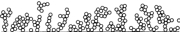
Figure 14 Final stage of simulation, Run 11. Simulation conditions: 0.2 packing density, 0.1 sticking probability, 1 pixel amplitude and 200 pixels to aggregate.
