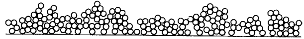
Figure 16 Final stage of simulation, Run 13. Simulation conditions: 0.2 packing density, 0.01 sticking probability, 10 pixels amplitude and 200 pixels to aggregate.
